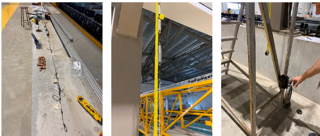
Fig. 12. Setup of Spring Combinations for Mooring Line testing.
